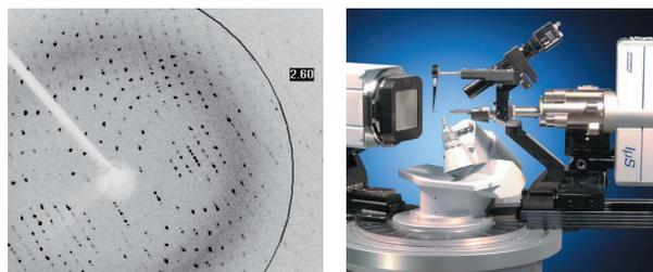
Figure 1: Diffraction pattern of the endothiapepsin crystal (left;  $15 \text{ s}/0.5^\circ$ ); X8 PROSPECTOR with a  $\text{Cu-}1\mu\text{S}$  microfocus X-ray source equipped with a QUAZAR MX optics and APEXII CCD detector (right).
